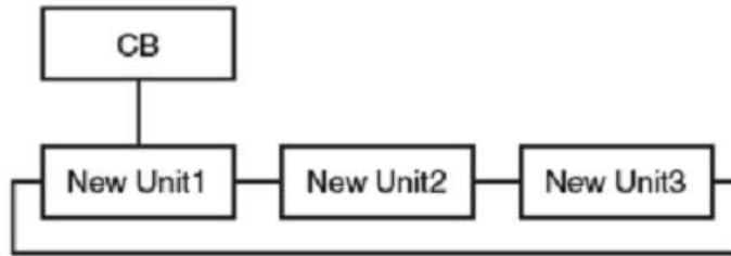
FIGURE 28 Case 1: Ring of potential PEs with one direct connection to the CB
